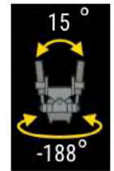
Auto Return Function Return to set rotate and tilt position of attachment connected below the TRS
