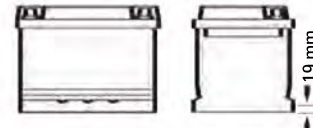
B4 Base holddown 19 mm (on long sides)
