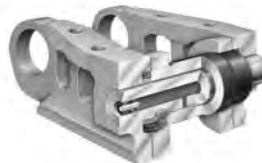
Sealed and Lubricated Track
