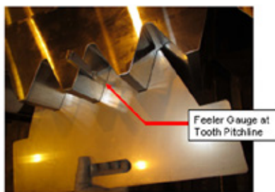
Figure 5 - Feeler Gauge Measurement at Gear Tooth Flank Pitchline (Center of Tooth)
