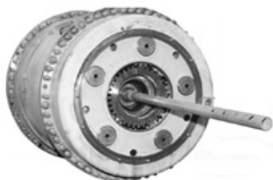
Installer attached to shaft (sling not shown)
